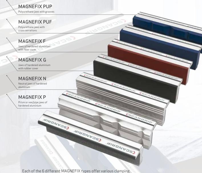
Each of the 6 different MAGNEFIX types offer various clamping abilities and are useful for different kinds of work. The jaws can also be used in combination. For instance, for taper pins or thin walled tubes use N or P together with G. For irregularly profiled parts with one flat surface use F on the flat surface and G on the profiled side.
